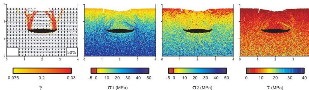
**Figure 3:** DEM model of pit crater or caldera collapse at 50% depletion. Plots show, from left to right, trajectories of maximum principal stress and values of maximum finite shear strain ( $\gamma$ ), as well as magnitudes of maximum principal stress ( $\sigma_1$ ), minimum principal stress ( $\sigma_2$ ), and maximum shear stress ( $\tau$ ). Magma reservoir particles are here coloured black.
