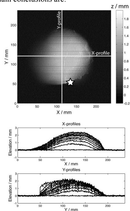
Fig. 2 – Top. Plot of the topographic data monitored during an experiment. The white star locates the eruption site. The white lines locate the corresponding topographic X- and Y-profiles. Bottom. Plots of the topographic profiles located on the maps. Each curve represents a transient stage of the model surface. The time step of monitoring between each profile was constant during each experiment (4s). Notice the vertical scale dilation.
