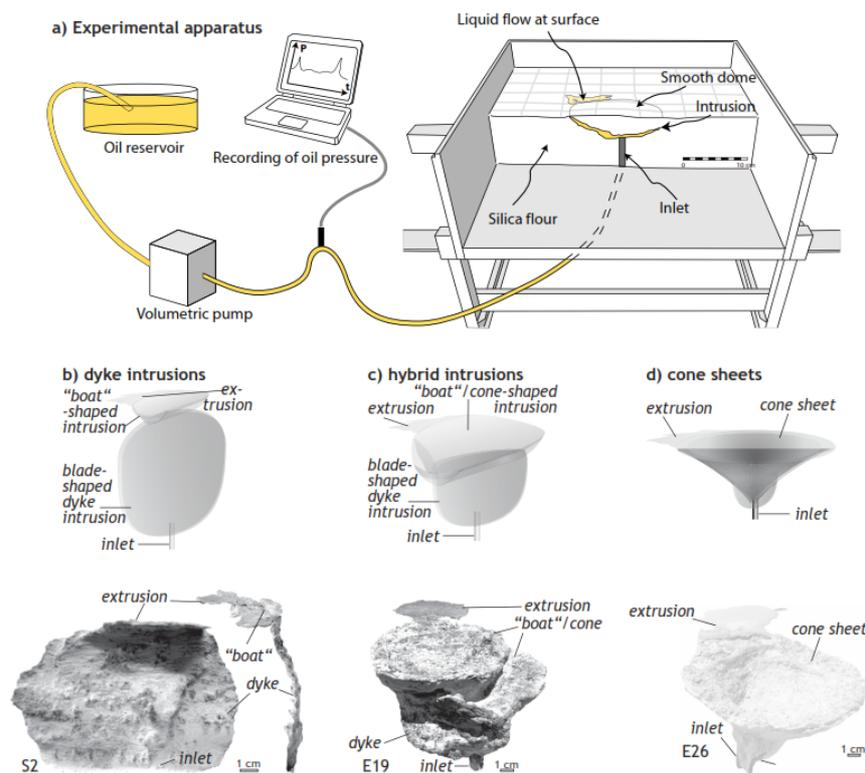
Figure 1. a) Sketch of the experimental setup of our experiments. b)-d) Sketches and photographs of experimentally-produced intrusions.
