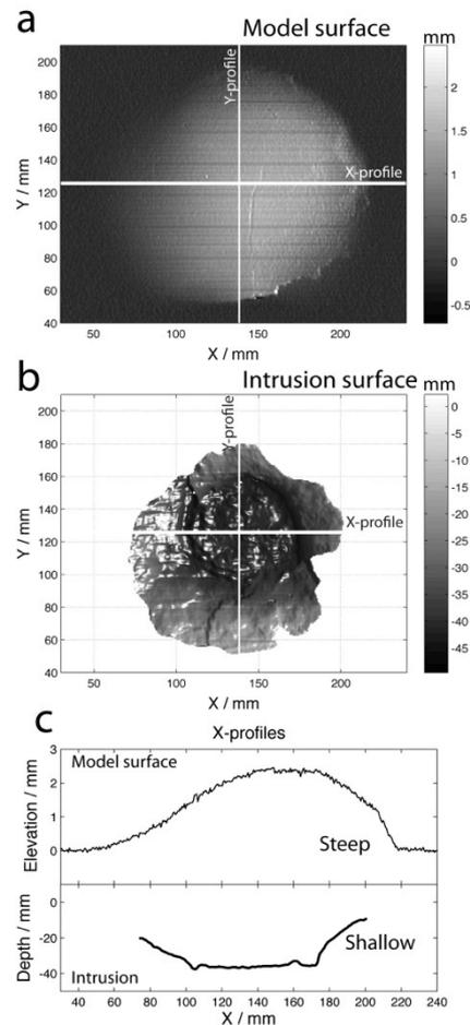
Fig. 4 – Topographic map of model surface before the eruption of the oil. b. Topographic map of the top surface of the excavated intrusion. Plots of topographic profiles of the model surface (top) and the underlying intrusion (down) parallel to the Y-axis (Y-profile).
