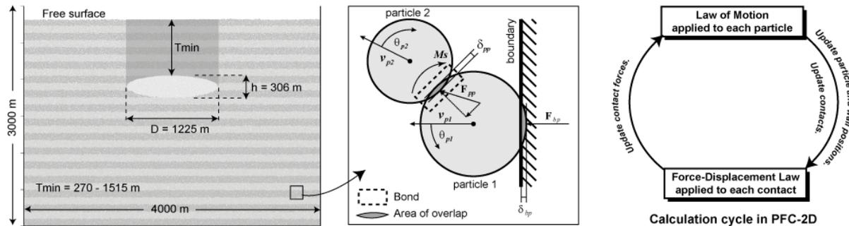
**Figure 1:** Overview of DEM as implemented in PFC-2D. **Left:** Pre-depletion view of a collapse caldera model. Boundary wall conditions are free-slip. **Centre:** Close up of particle-bond-wall relations. **Right:** Schematic of PFC calculation cycle.
