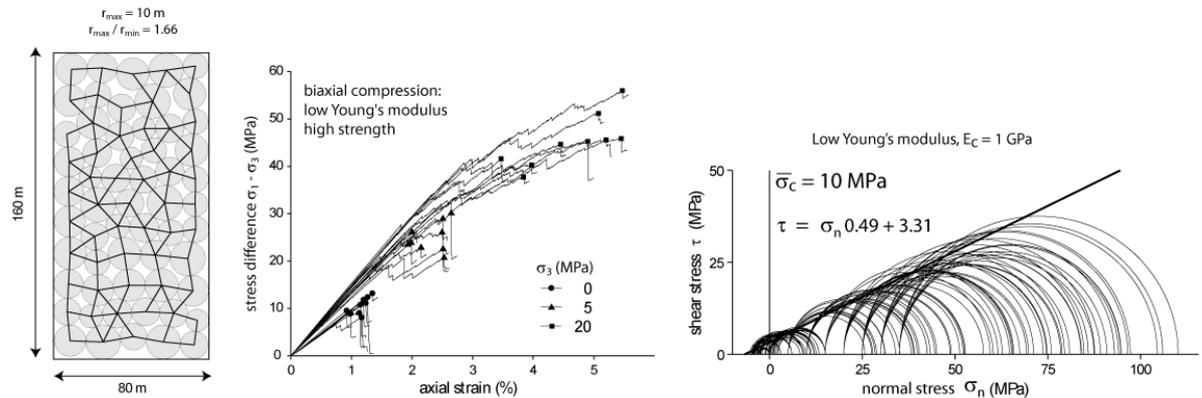
**Figure 2:** Bulk property calibration in DEM models. **Left:** Sample of model subject to biaxial compression and tension tests. **Centre:** Stress-strain plot for biaxial compression at various confining pressures, each with 10 realisations. Symbols on curves denote peak strengths. Post-peak curves are removed for clarity. **Right:** Compression test results fitted to a Mohr-Coulomb failure envelope.
