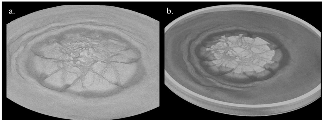
**Figure 1.** Reconstructed 3D volume of a low cohesion sand cone from X-ray scan after 72 h of gravitational spreading over a 4.5 mm silicone layer. The cone is 7.9 cm in diameter, and 1 cm high. (a) Oblique 3D view of model surface with 100  $\mu\text{m}$  spatial resolution; (b) virtual horizontal cross section at mid-height through the cone, showing radial pattern of graben-bounding faults as low density dark areas (from Kervyn et al. 2010).
