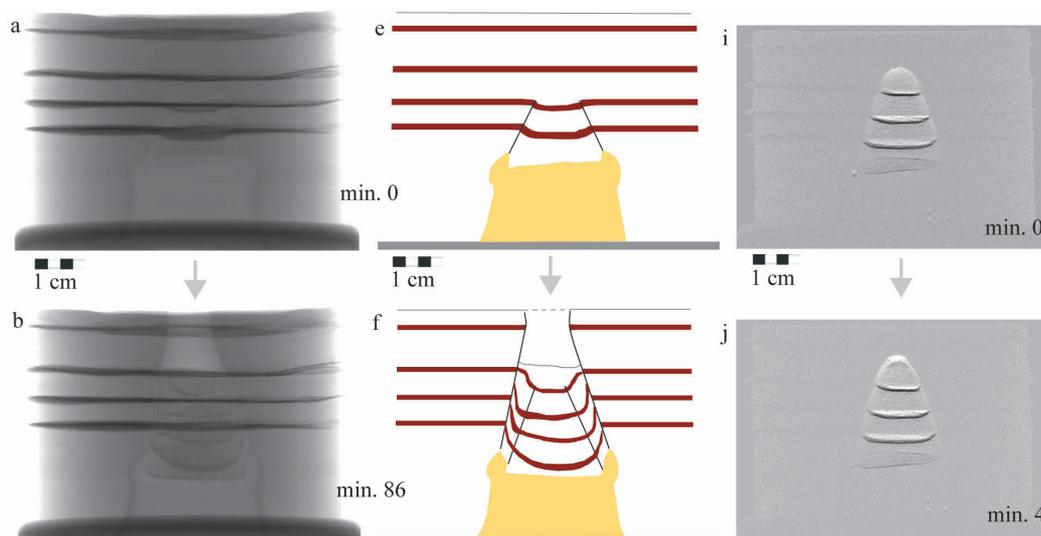
**Figure 2:** a. Radiograph sequence acquired during GS drainage in caldera collapse model, at H/D equal to  $\sim 0.8$ ; b. structures observed in the radiographs (red: garnet sand, yellow: golden syrup); c. Radiograph difference image, highlighting increase (black) or decrease (white) in material density (from Poppe et al. in prep).
