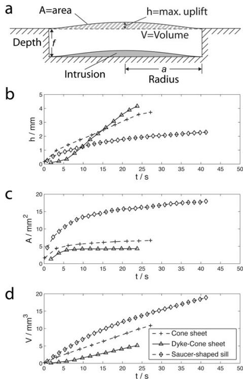
Fig. 3 – a. Sketch describing the maximum uplift  $h$  (mm), area  $A$  (mm<sup>2</sup>), and uplifted volume  $V$  (mm<sup>3</sup>). b,c,d. Plots of  $h$ ,  $A$ , and  $V$  as a function of time  $t$  (s). Crosses represent experiment with cone sheet, triangles represent experiment with dyke-to-cone sheet, and diamonds represent experiment with saucer-shaped sill.
