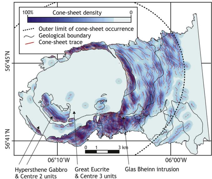
**Fig. 4.** Map displaying the traces of Ardnamurchan cone-sheets and their distribution density using a density grid with a resolution of 20 m. A relative density scale is used, with density values ranging from 0 to 100%. Data are based on the geological map and associated field notes (Emeleus, 2009) and represent minimum numbers of minor intrusions per area.
