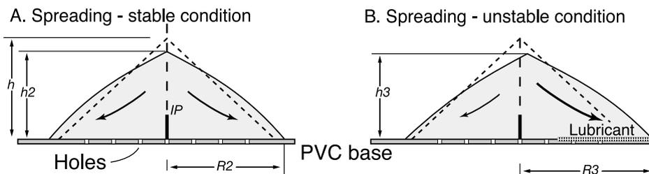
Fig. 4. Geometry of experimental cones in stable situation (A) and unstable situation (B). Due to gravity, the cones spread outward, partially sliding on a basal lubricant. In the unstable situation, only one flank was lubricated. IP, injection point (10 mm above base), basal radii  $R_3 > R_2 > R_1$ ; cone height  $h > h_2 > h_3$ . Through small holes drilled in the basal plate, injection was possible at various positions.
