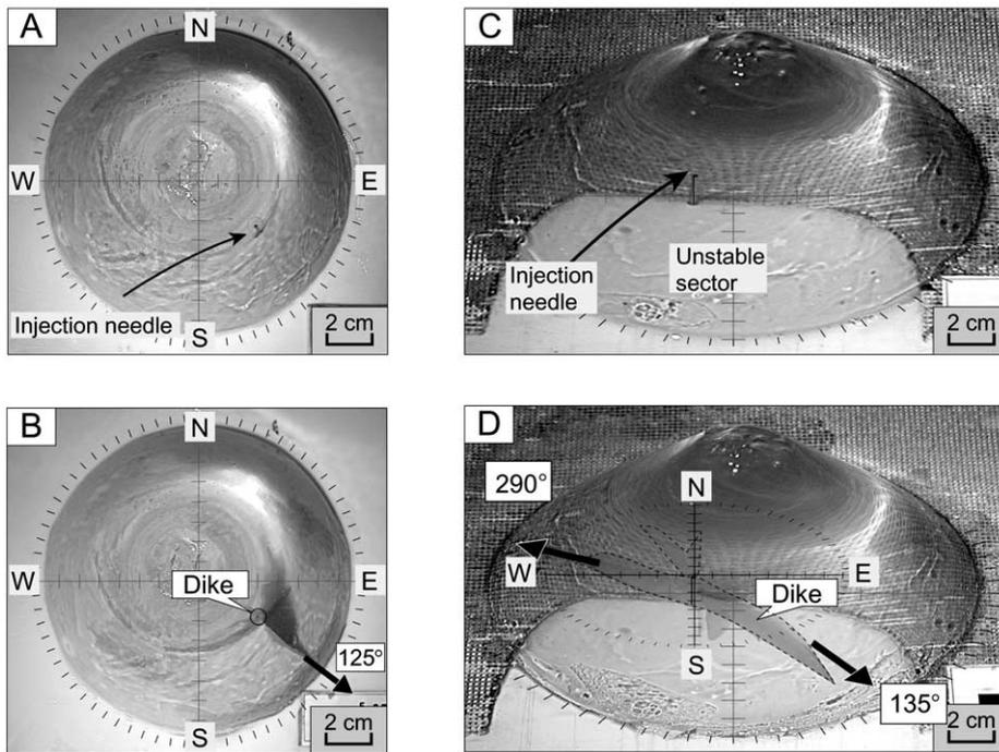
Fig. 5. Photographs of experiments before (panels A and C) and after injection (panels B and D). (A) Plan view of stable situation, forming (B) a radial dike oriented  $125^\circ$  azimuth on injection. (C) Oblique view of unstable situation with injection into the interface creeping/non-creeping sector and a slight southwestward eccentricity of the lubricated base. (D) Produced fractures to southeast ( $135^\circ$ ) and northwest ( $290^\circ$ ).
