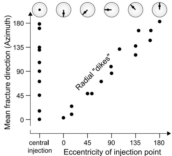
Fig. 6. Stable situation: Relation of mean hydro-fracture propagation direction to the eccentricity of the injection point (measured in azimuth). Situated on a uniform substratum, the flanks of the gelatin cone deformed by gravity-driven extension only. Central injection beneath the apex of a regular cone generates randomly directed fractures. Injection into the cone flanks produces fractures oriented radially, i.e. away from the edifice center.
